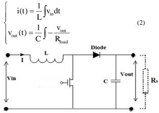
Figure 2: The boost DC/DC converter
